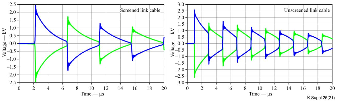
**Figure 4 – Magnetically coupled surge voltages at link ends for screened and unscreened cable (terminated 1 km link end voltages — blue and green lines)**
