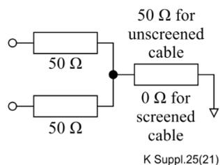
**Figure 3 – Signal terminating network for an SPE link cable**
