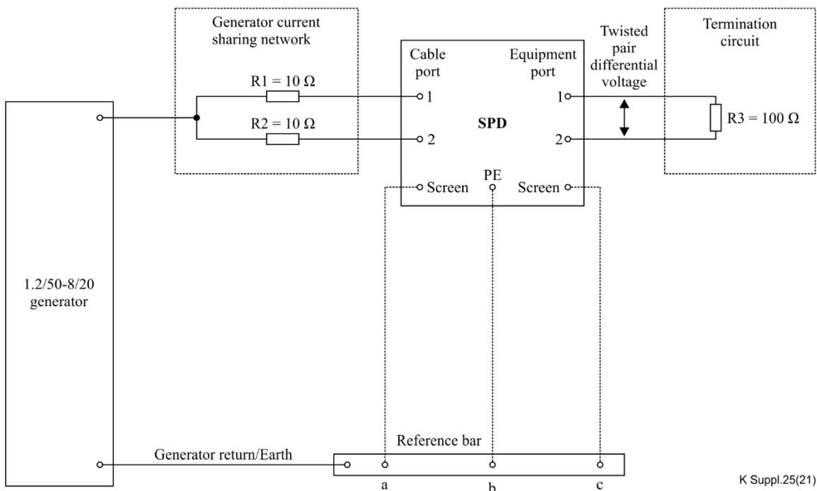
**Figure 12 – Twisted-pair common-mode to differential mode voltage surge conversion test circuit**
