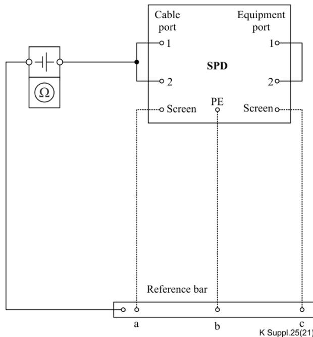
**Figure 14 – Test circuit to measure the insulation resistance of an SPD with a PE terminal or screen terminals, or both**
