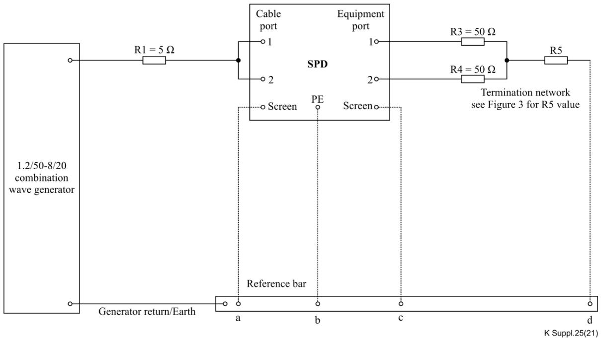
**Figure 9 – Impulse limiting voltage under common-mode surge conditions**
