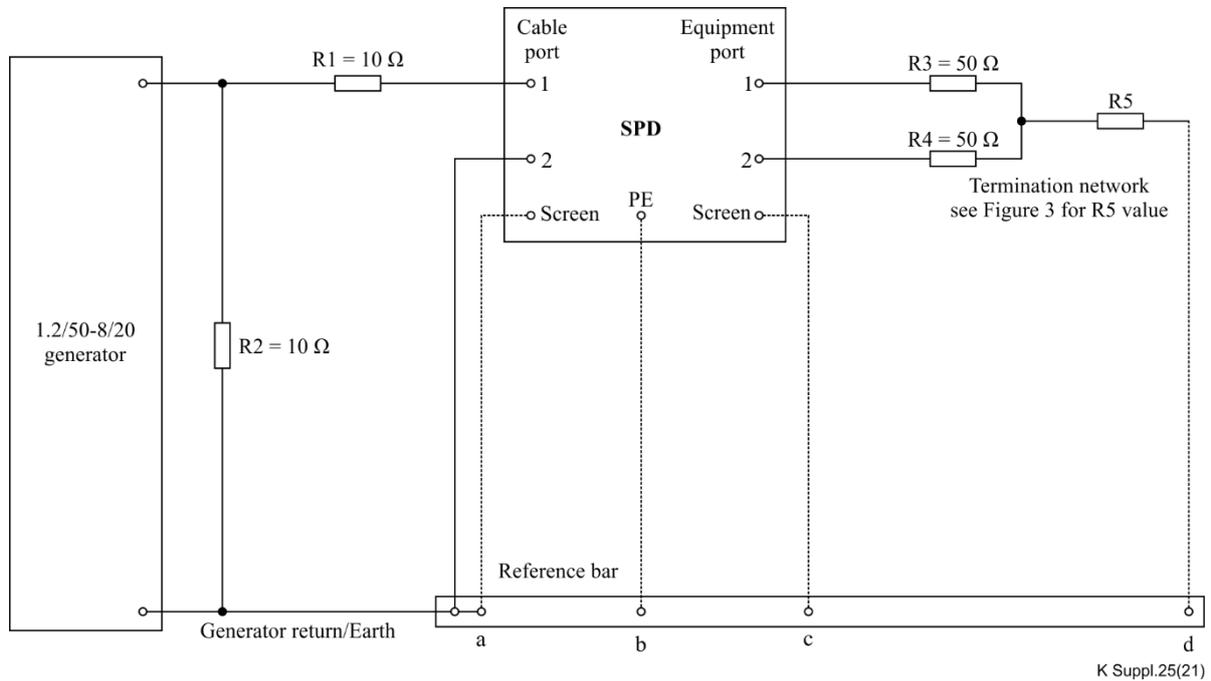
**Figure 10 – Single twisted-pair differential-mode surge test circuit**
