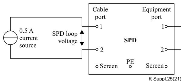
**Figure 15 – Test circuit to measure the PoE SPD d.c. input/output voltage drop**
