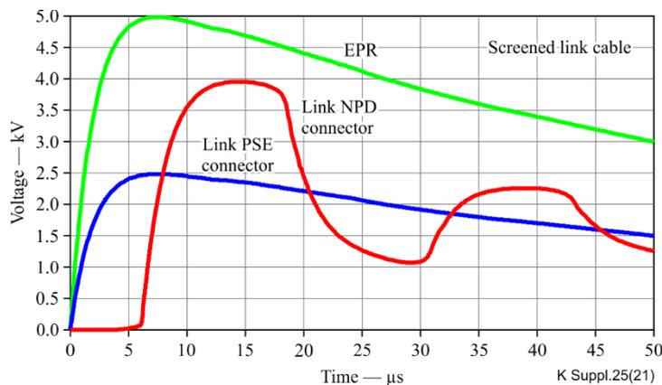
**Figure 6 – PSE differential-mode choke EPR link voltage reduction (5 kV EPR — green line; reduced to 2.5 kV at the PSE link connector – blue line; results in 4 kV – red line)**
