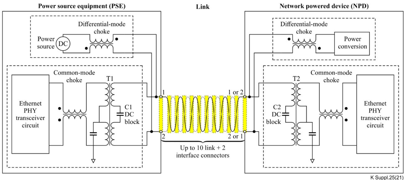
**Figure 1 – Basic 10 Mb/s, 1 km SPE system arrangement providing both Ethernet data and powering**
