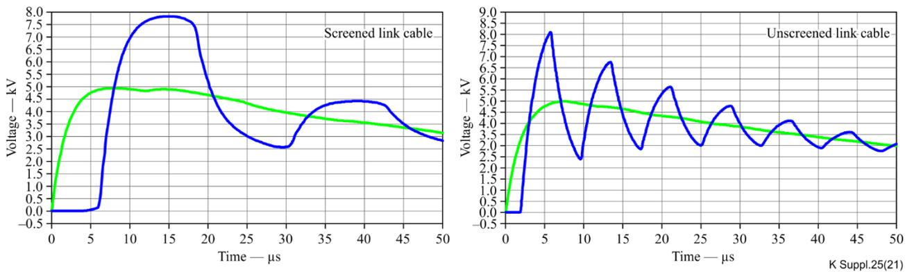
**Figure 5 – 5 kV peak earth potential rise at one link end produces some 8 kV at the other link end (EPR – green line; NPD – blue line)**
