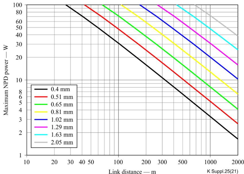
**Figure 7 – Maximum NPD power versus distance for various wire diameters (based on a nominal 54 V PSE)**
