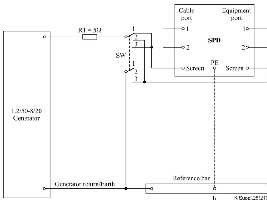
**Figure 13 – Screen bonding test**
