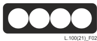
Figure 2 – Cross-section of a typical encapsulated ribbon
