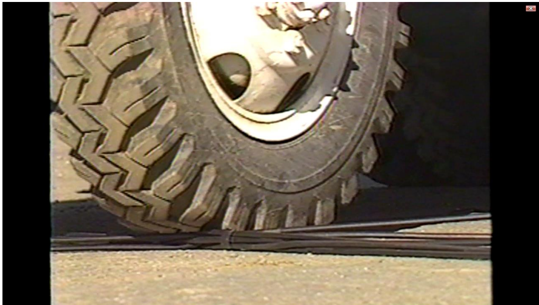
Figure I.5 – Abusive testing of central core, linear strength member, armoured sheath
