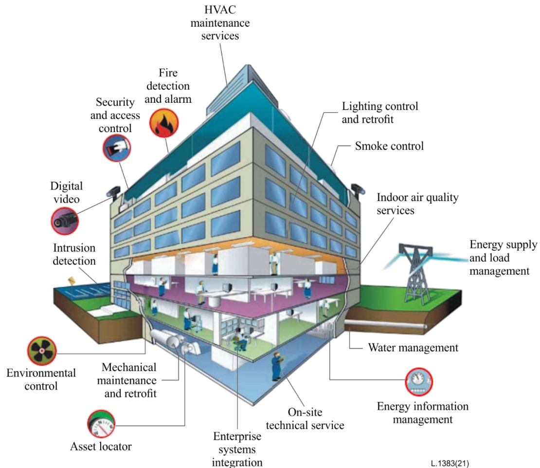
Figure 1 – Smart Energy in a Business Building (the elements shown are applicable to buildings in business districts such as offices and malls)
