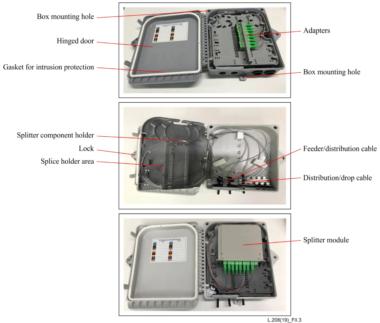
Figure II.3 – Typical examples of fibre distribution boxes used as FDH and MDUB for low fibre density applications
