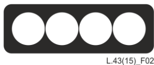
Figure 2 – Cross-section of a typical encapsulated ribbon
