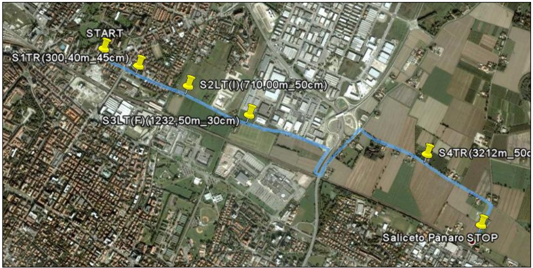
Figure I.2 – GPR data imported in GIS system
