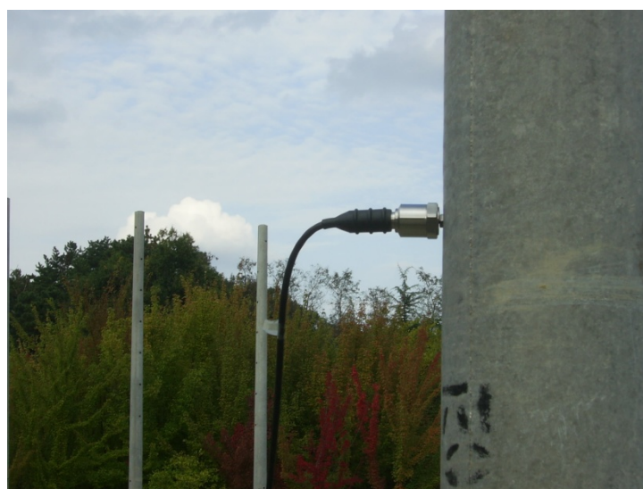
Figure II.2 – Accelerometer used in the test
