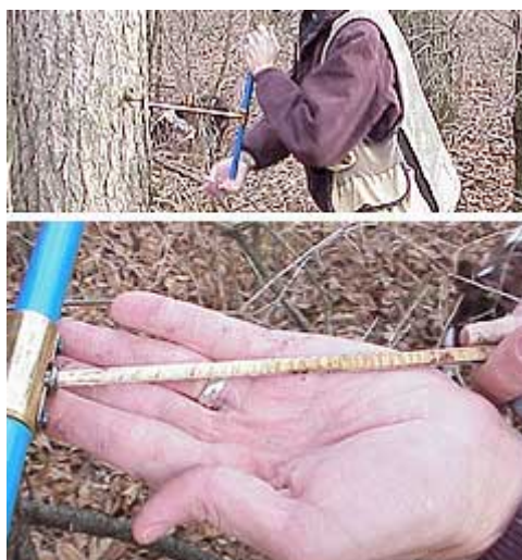
Figure 1 – Operation with the drill probe
