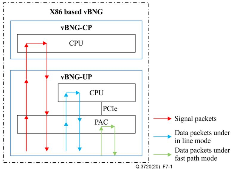
**Figure 7-1 – Illustration of packet flow paths for two working modes**
