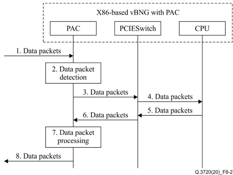
**Figure 8-2 – Procedure for processing data packets in in-line mode**
