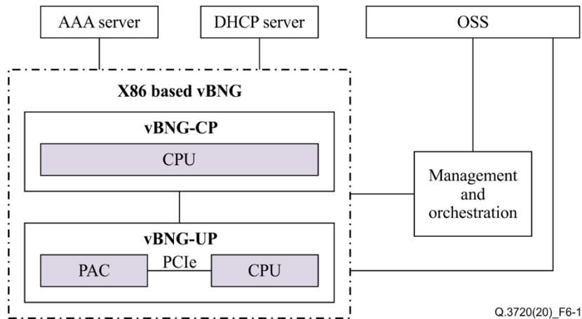
**Figure 6-1 – Framework for X86-based vBNG acceleration with PAC**
