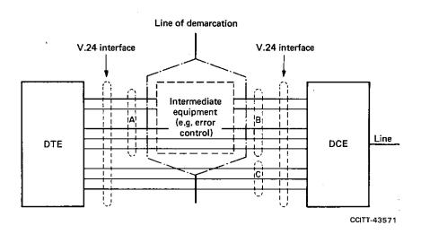
Without intermediate equipment the selections A and B are identical. Selection C may be a selection specifically for automatic calling.
