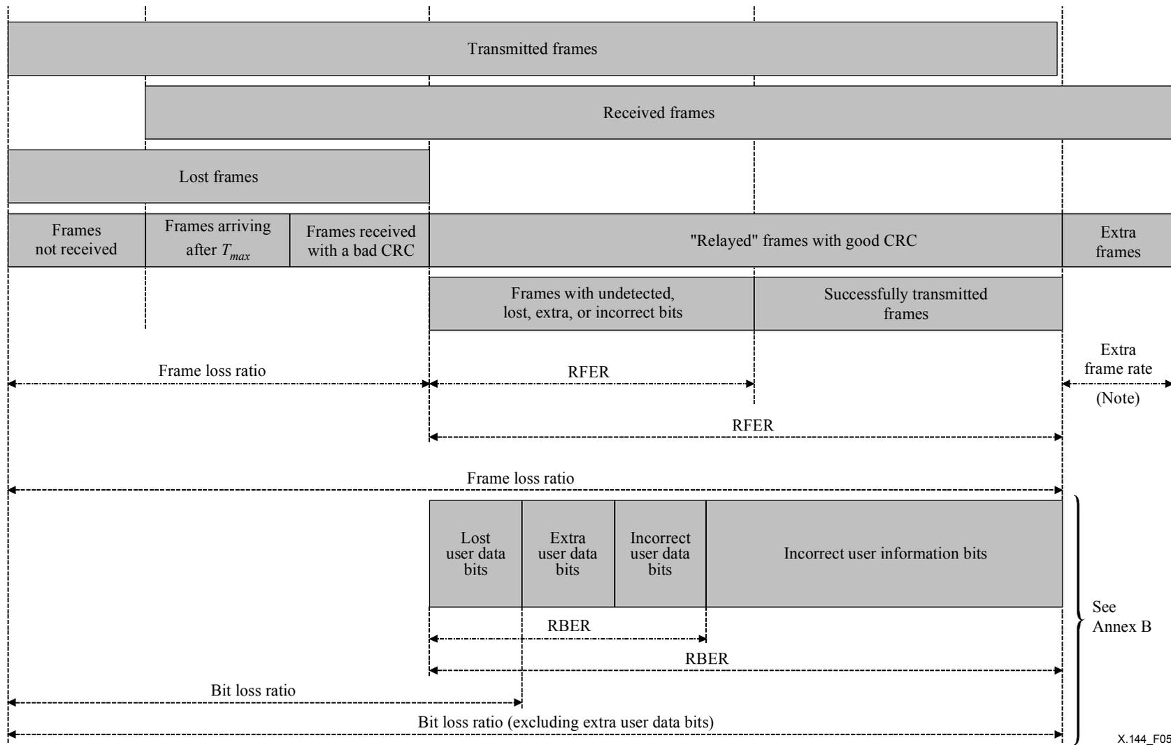
**Figure 5/X.144 – Statistical populations used in defining selected accuracy and dependability parameters**
