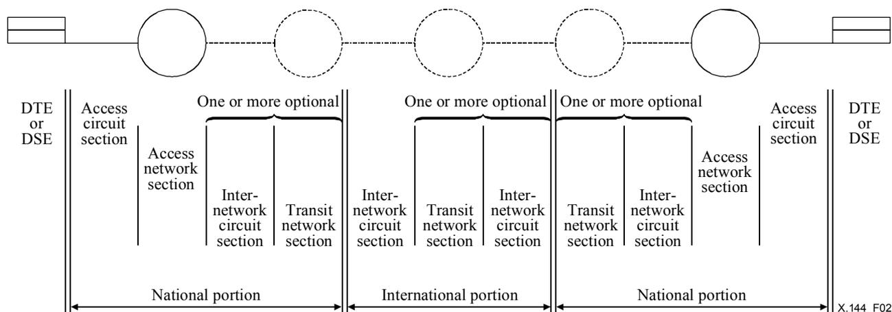
**Figure 2/X.144 – Sections of an international virtual connection**
