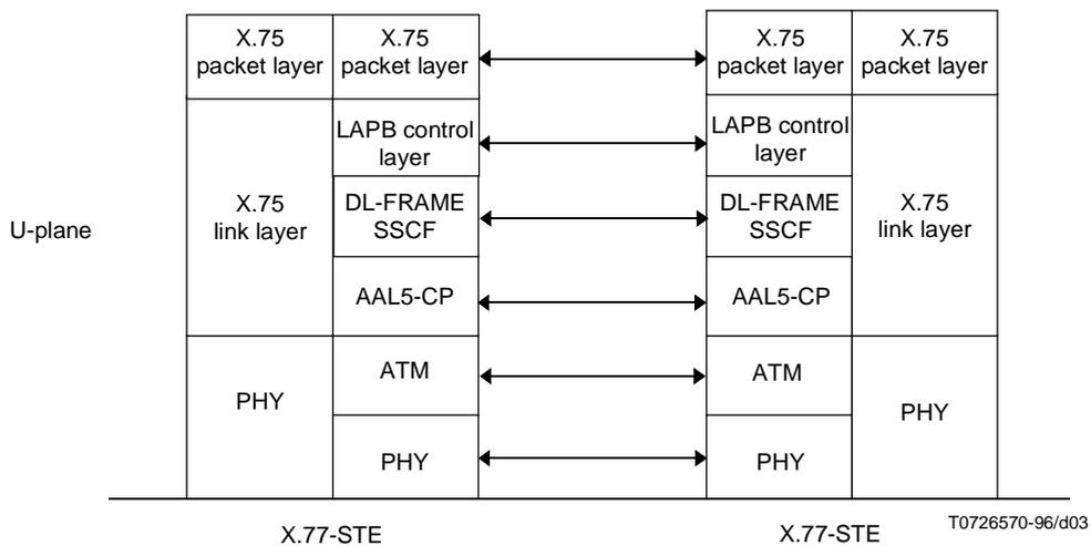
NOTE – X.75 or some equivalent internal network protocols. This figure shows the protocol stack where X.75 is used here.
