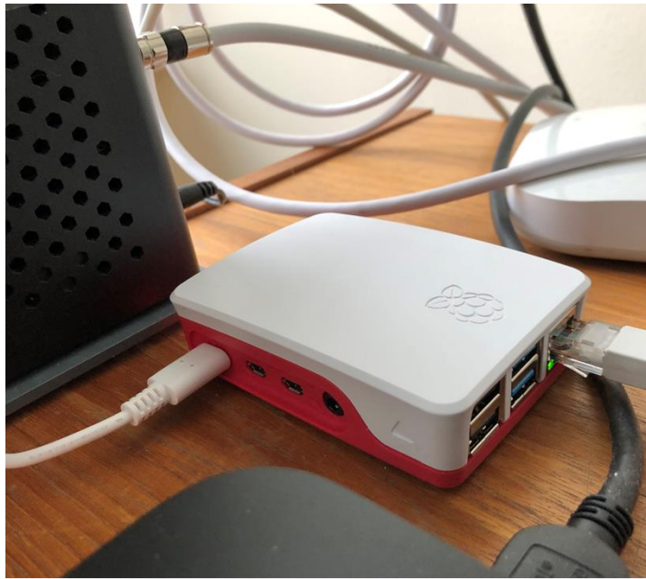
Figure 9-5 – Raspberry Pi 4 Model B running udpst 7.1 client as baremetal host
