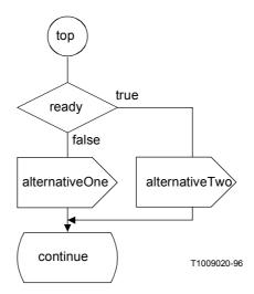
Note that the pointlist for the flowline after the output symbol alternative Two has four points, two of them on the border of symbols.
