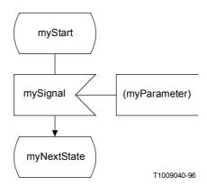
Note that the text extension line is described as if its endpoints were on the border of the surrounding rectangles of the attached symbols even if this is not completely true in GR. (The endpoint on the input symbol is inside the surrounding rectangle.) This rule applies to all lines/channels connected to symbols that are not rectangular shaped. (Stop symbol, process symbol...)
