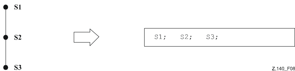
Figure 8/Z.140 – Illustration of sequential behaviour
