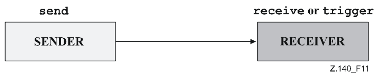
Figure 11/Z.140 – Illustration of the asynchronous send and receive
