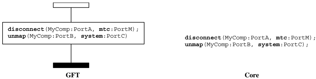
Figure 43/Z.142 – Disconnect and unmap operation
