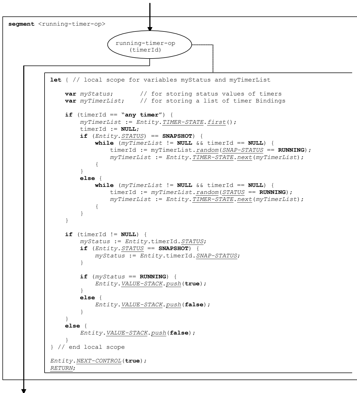
Figure 114 – Flow graph segment <running-timer-op>
